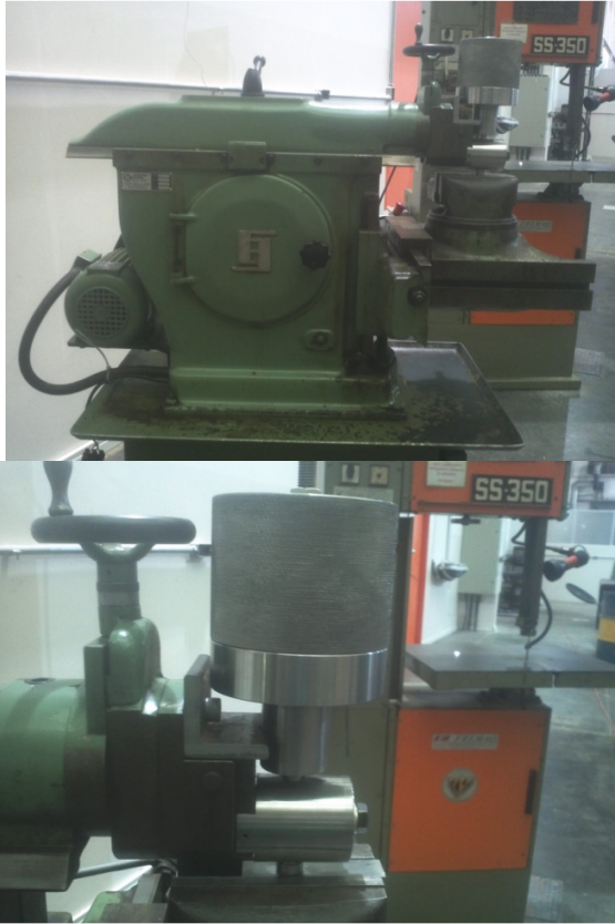
Figure 13 – Test equipment with 10 kgf load.
