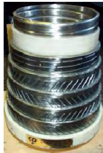
Figure 2 – Flexible pipe, [LEMOS, 2005].
